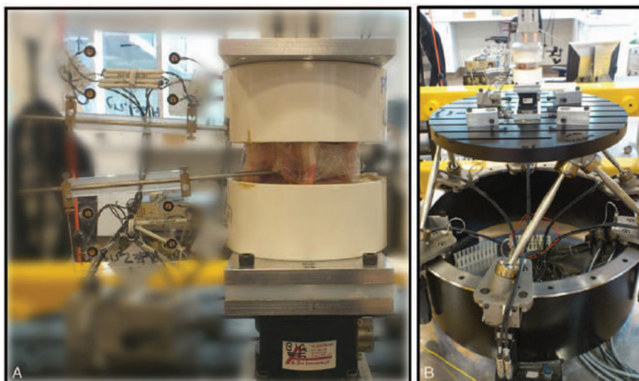
Figure 3. Robotic testing. (A) Potted specimen with L4 mounted to the six-axis load cell and L3 fixed to a stationary cross beam. (B) Parallel robot platform with load cell and specimen attached.
