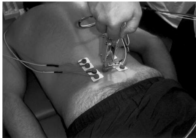
Figure 1. The experimental setup for a spinal manipulative thrust applied over the L4 spinous process. The hand-held spinal manipulation device, the Activator Adjusting Instrument, equipped with an impedance head and preload control frame, is shown with its 1 cm 80-durometer rubber tip attached to the end contacting the patient. The device is manually activated by means of a spring mechanism that propels a hammer into a stylus producing an approximate 150 N force in about 5 msec. Electrode placement adjacent to the L3 and L5 functional spinal units is shown.
